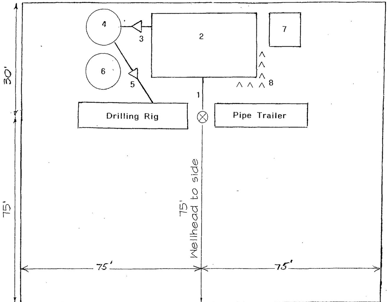
Closed Loop Drilling System
