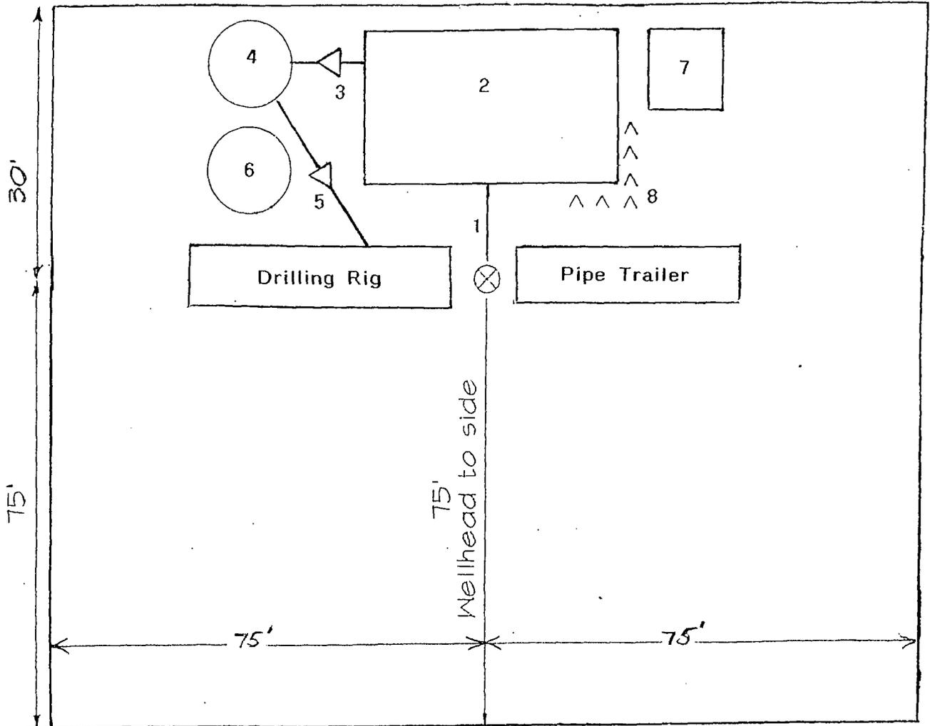
Closed Loop Drilling System
