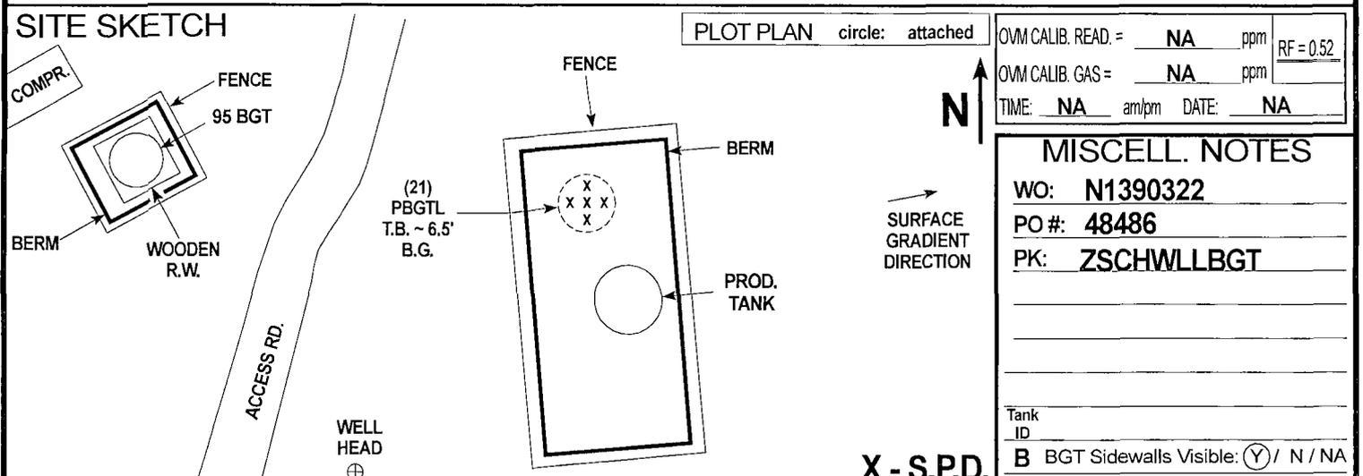
NOTES: BGT = BELOW-GRADE TANK; E.D. = EXCAVATION DEPRESSION; B.G. = BELOW GRADE; B = BELOW; T.H. = TEST HOLE; ~ = APPROX.; T.B. = TANK BOTTOM; PBGTL = PREVIOUS BELOW-GRADE TANK LOCATION; SPD = SAMPLE POINT DESIGNATION; R.W. = RETAINING WALL; NA = NOT APPLICABLE OR NOT AVAILABLE; SW - SINGLE WALL; DW - DOUBLE WALL; SB - SINGLE BOTTOM; DB - DOUBLE BOTTOM.
