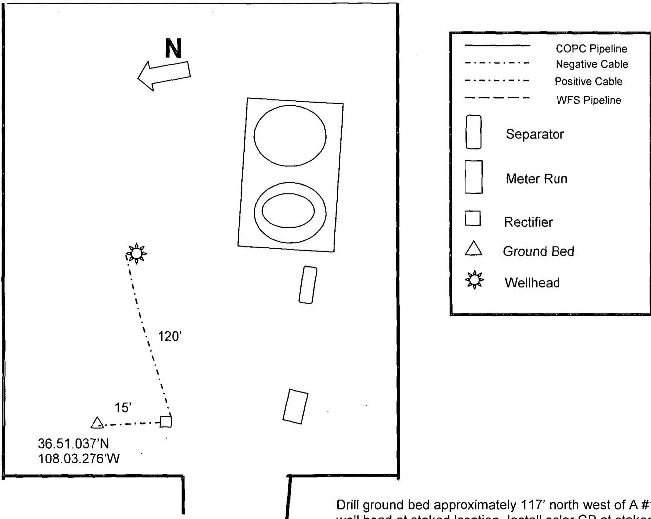
Drill ground bed approximately 117' north west of A #1E well head at staked location. Install solar CP at staked location. Install cable to new ground bed and to A #1E wellheads at lengths below.
