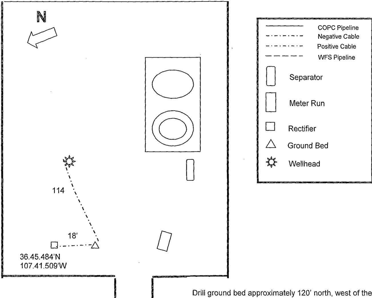
Drill ground bed approximately 120' north, west of the #1M well head at staked location. Install single well solar CP at staked location. Install cable to new ground bed and to the #1M wellheads at lengths below.
