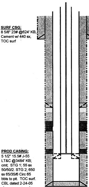
2 3/8" Tubing @ +/- 3420' 1 1/4" x 16' polished rod 3/4" rods 2'X1 1/2"X12' RWAC pump
