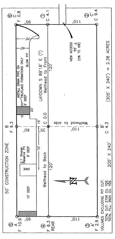
RESERVE PIT DIKE: TO BE 8' ABOVE DEEP SIDE (OVERFLOW — 3' WIDE AND 1' ABOVE SHALLOW SIDE). BLOW PIT: OVERFLOW PIPE HALFWAY BETWEEN TOP AND BOTTOM AND TO EXTEND OVER PLASTIC LINER AND INTO BLOW PIT.
