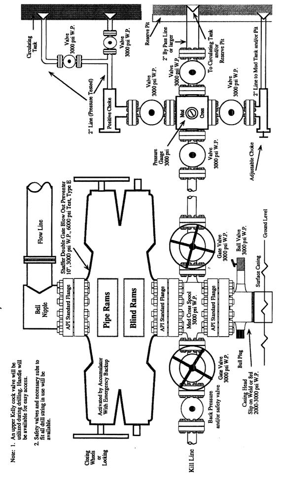
Note: This equipment is designed to meet requirements for a 2-M rating standard per 43 CFR part 3160 (amended). Proper operation and testing of equipment will be carried out per standard. 2,000 psi equipment can be substituted in the drawing to meet minimum requirements per standard.
