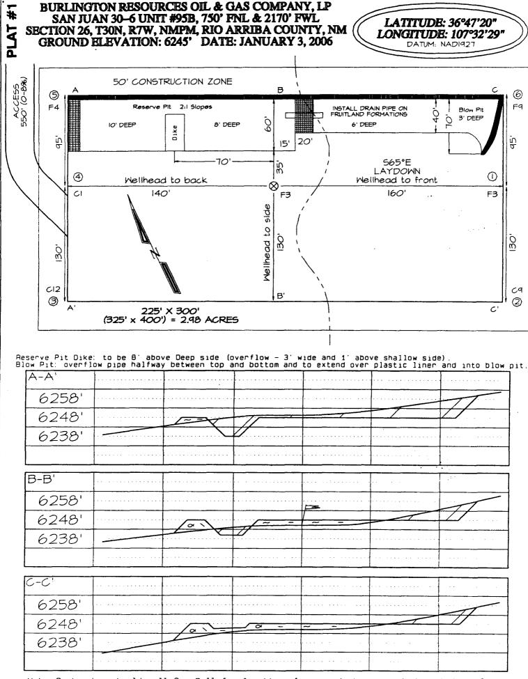
Note: Contractor should call One-Call for location of any marked or unmarked puried pipelines or cables on well pad and/or access road at least two (2) working days prior to construction
