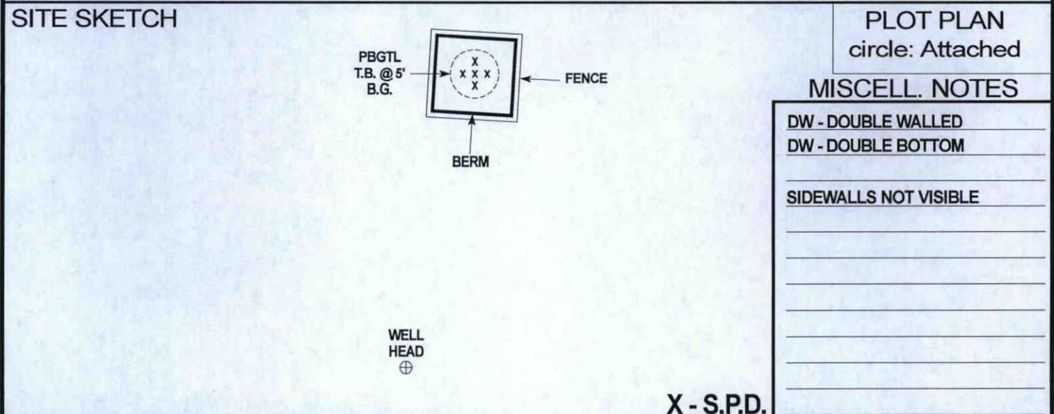
NOTES: BGT = BELOW-GRADE TANK; E.D. = EXCAVATION DEPRESSION; B.G. = BELOW GRADE; B = BELOW; T.H. = TEST HOLE; ~ = APPROX.; T.B. = TANK BOTTOM; PBGTL = PREVIOUS BELOW-GRADE TANK LOCATION; SPD = SAMPLE POINT DESIGNATION; R.W. = RETAINING WALL. MAGNETIC DECLINATION @ 13.5°E
