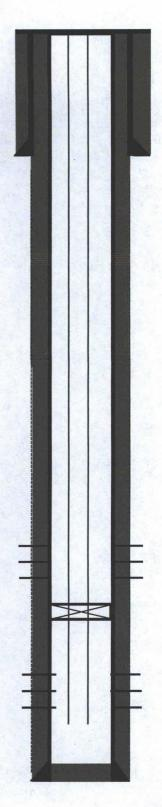
7"·23# ST & C casing @ 125'. Circulated cement to surface
