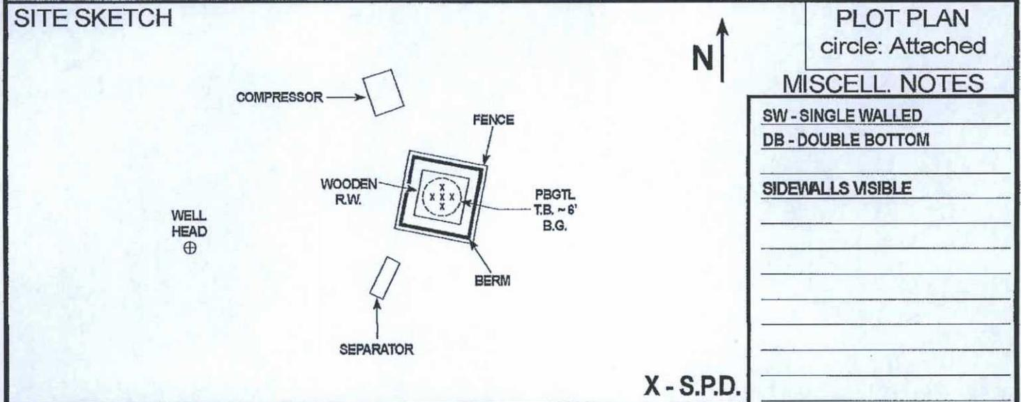
NOTES: BGT = BELOW-GRADE TANK; E.D. = EXCAVATION DEPRESSION; B.G. = BELOW GRADE; B = BELOW; T.H. = TEST HOLE; ~ = APPROX.; T.B. = TANK BOTTOM; PBGTL = PREVIOUS BELOW-GRADE TANK LOCATION; SPD = SAMPLE POINT DESIGNATION; R.W. = RETAINING WALL
