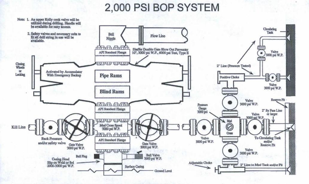
Note: This equipment is designed to meet requirements for a 2-M rating standard per 43 CFR part 3160 (amended). Proper operation and testing of equipment will be carried out per standard. 2,000 psi equipment can be substituted in the drawing to meet minimum requirements per standard.
