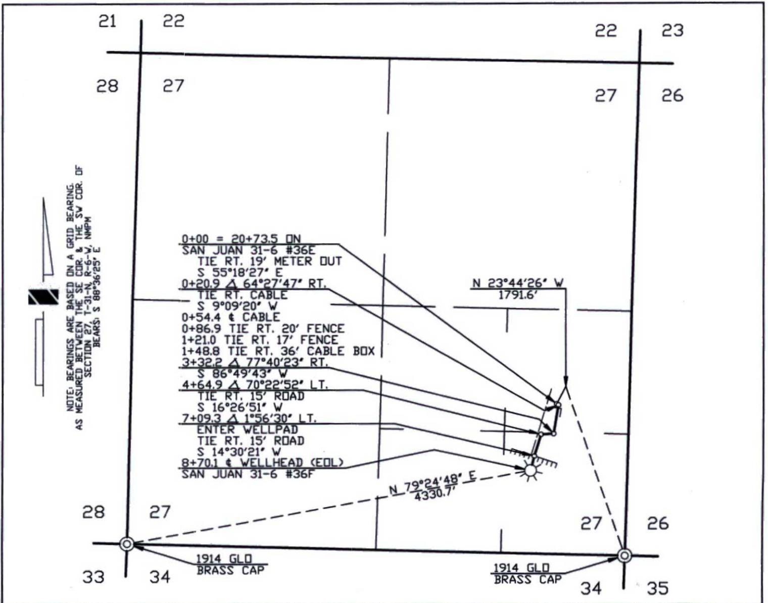
NOTE: BEARINGS ARE BASED ON A GRID BEARING. AS MEASURED BETWEEN THE SE COR. & THE SW COR. OF SECTION 27, T-31-N, R-6-W, NMPM BEARS: S 88°36'25" E
