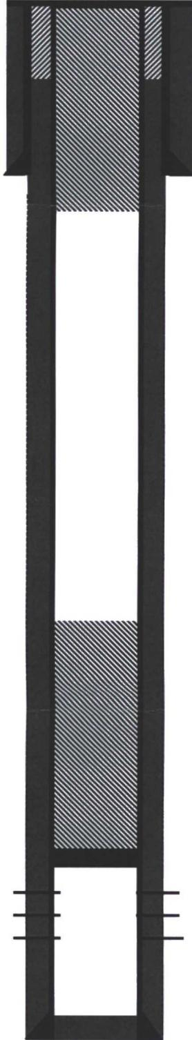
7" 20# ST & C casing @ 94'. Cemented w/ 35
