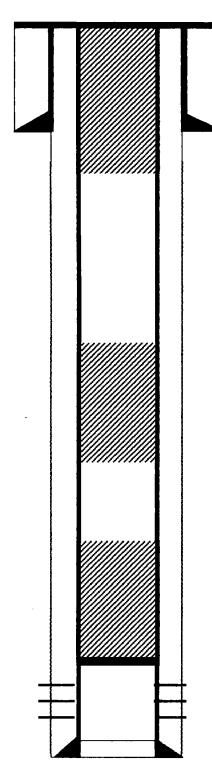
$7^{\prime\prime}$  J-55 23# casing @ 120'. Cemented with 50 sks Class B. Hole size 9-1/8"
