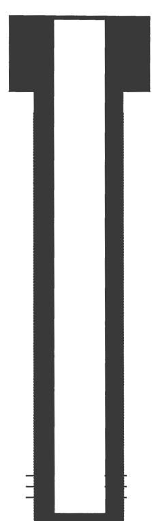
$7^{\prime\prime}$  J-55 23# casing @ 120'. Cemented with 50 sks Class B. Hole size  $9\text{-}1/8^{\prime\prime}$
