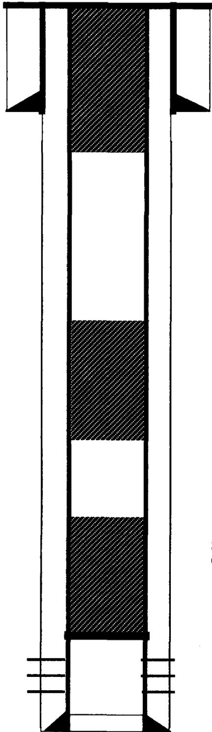
7" J-55 23# casing @ 120'. Cemented with 50 sks Class B.
