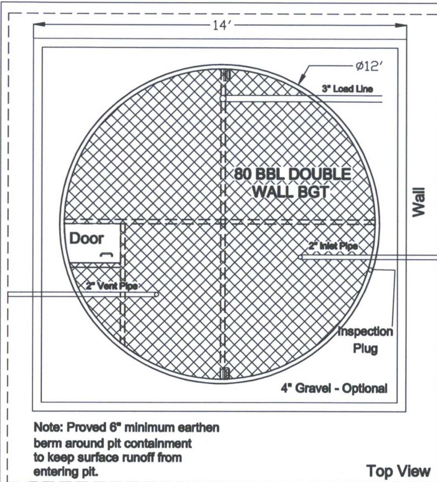
Note: Proved 6" minimum earthen berm around pit containment to keep surface runoff from entering pit.
