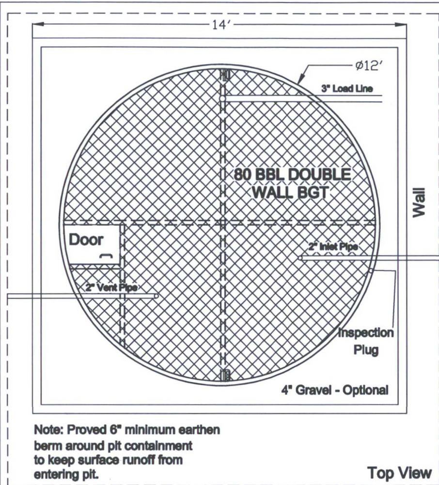
Note: Provide 6" minimum earthen berm around pit containment to keep surface runoff from entering pit.
