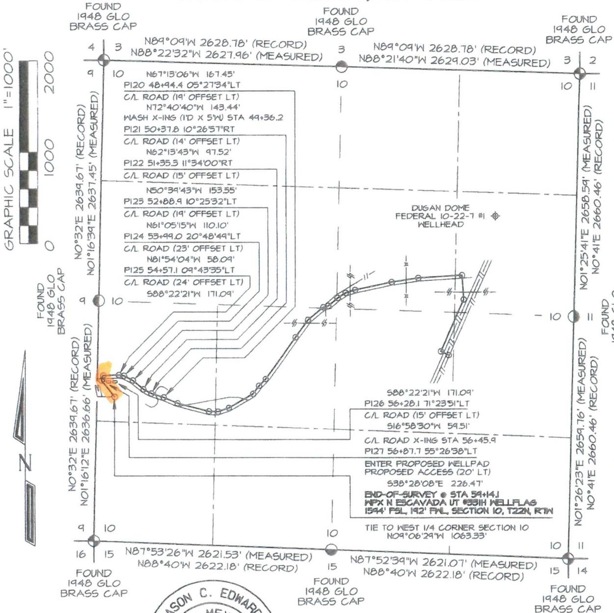
REAL-TIME KINEMATIC GPS SURVEY SOLUTION OBTAINED FROM SATELLITES TRACKED ON JULY 28, 2015 FROM A REFERENCE STATION POSITIONED IN SE/4 NW/4 OF SECTION 2, T22N, R7W
