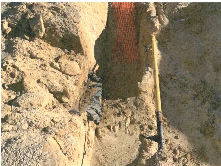
Photo 6: Buried liner near pump jack, suspected to be historic reserve pit.
