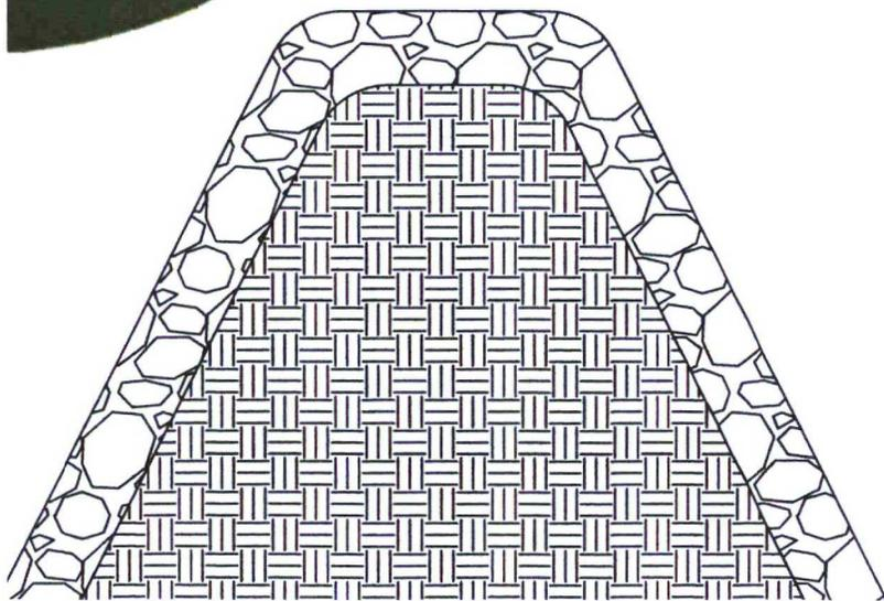
PROPERLY CONSTRUCTED FOUNDATION CONSISTING OF A LEVEL FREE OF ROCKS, DEBRIS, SHARP EDGES OR IRREGULARITIES T PUNCTURES CRACKS OR INDENTATIONS TO THE TANK BOTTOM.
