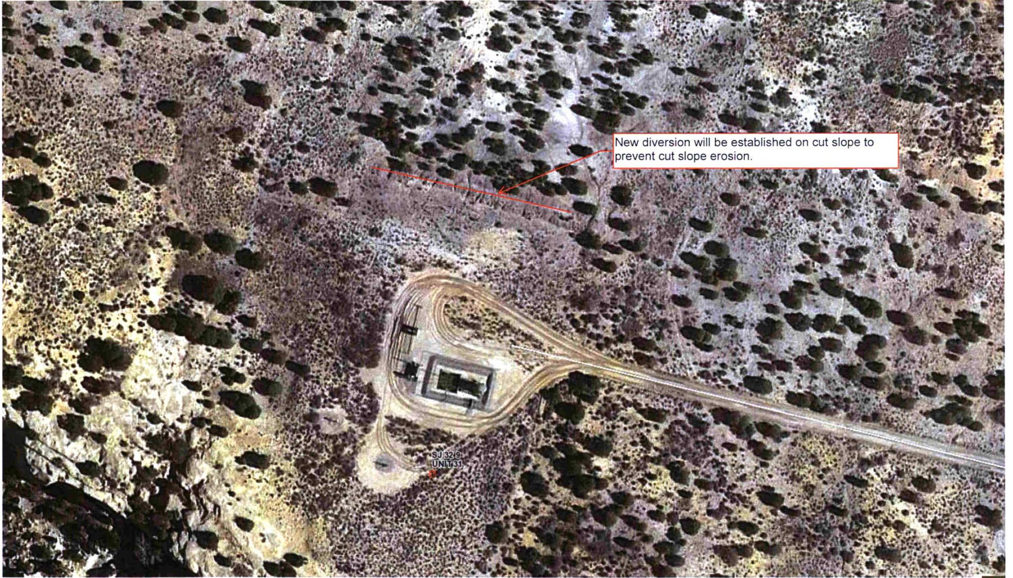
New diversion will be established on cut slope to prevent cut slope erosion.
