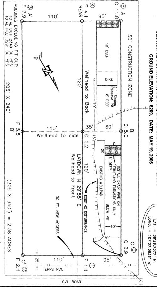
RESERVE PIT DIKE: TO BE 8' ABOVE DEEP SIDE BLOW PIT: OVERFLOW PIPE HALFWAY BETWEEN TOP (OVERFLOW - 3' AND BOTTOM AND TO EXTEND OVER PLASTIC LINER AND INTO BLOW PIT. WIDE AND 1' ABOVE SHALLOW SIDE)
