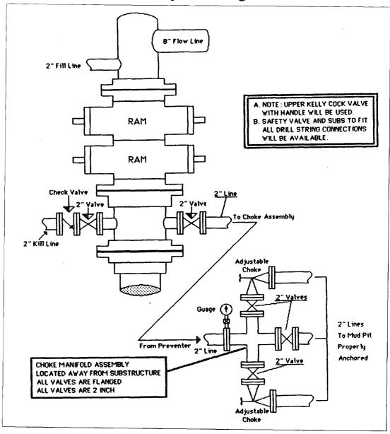
A BOP Stack consisting of either a manual two(2) ram preventer, (double or 2 singles) or a single Hydraulic annular preventer with a minimum of 1000 psi working pressure. The upper ram cavity Shall contain pipe rams to fit the drill pipe in use. The lower cavity shall contain blind rams.
