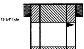
9-5/8" 25.4#, Casing set @ 132' Cement with 100 sxs, Circulated to Surface
