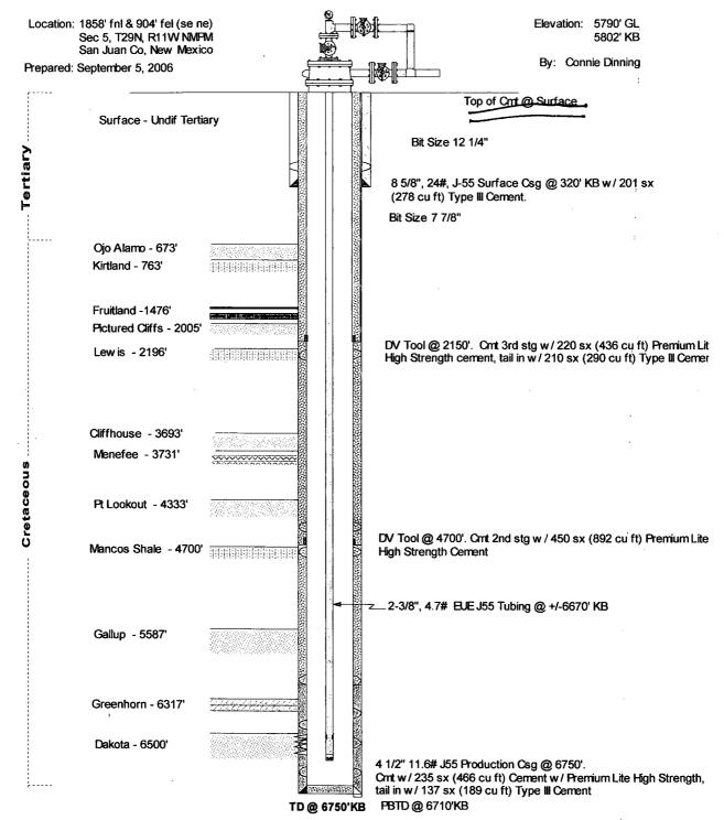
4-1/2" capacity = .0155 Bbl/ft 2-3/8" capacity = .00387 bbl/ft Annular capacity = .0101 bbl/ft
