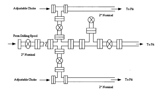
Choke manifold installed from surface to TD
