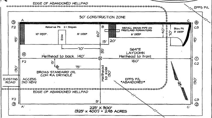
Reserve Pit Dike: to be 8' above Deep side (overflow - 3' wide and 1' above shallow side). Blow Pit: overflow pipe halfway between top and bottom and to extend over plastic liner and into blow pit.
