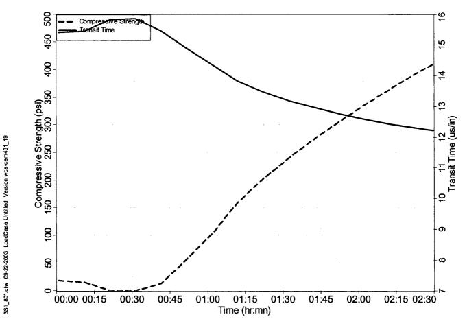
Lead Slurry Density = 15.80 lb/gal Time to 500 psi= 03:08 hr:mn Time to 1000 psi= 08:02 hr:mn
