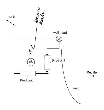
\*Revised 07-03 06-12-03 Removed Dehy Installed Prod Unit
