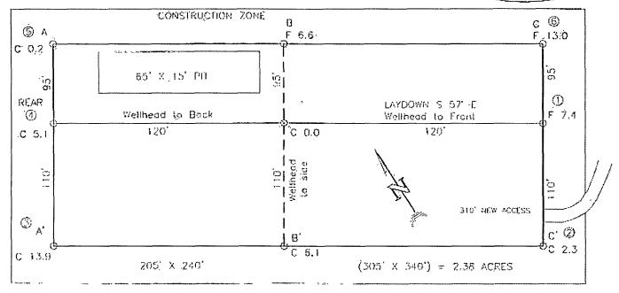
RESERVE PUT DIRE TO BE 8' ABOVE DEEP SIDE (CVERFLOW - 3' WIDE AND I' ABOVE SHALLOW SIDE) BLOW PIE: OVERFLOW PIPE HALFWAY BETWEEN TOP AND BOTTOM AND TO EXTEND OVER PLASTIC LIGHT AND INTO BLOW PIT.
