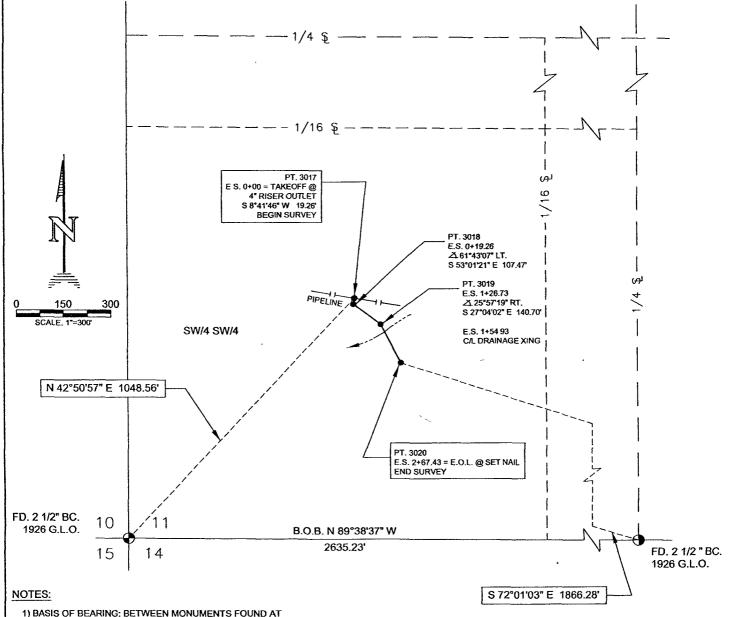
THE SOUTH QUARTER CORNER AND THE SOUTHWEST CORNER OF SEC. 11, T30N, R16W, N.M.P.M. LINE BEARS N 89°38'37" W A DISTANCE OF 2635.23' PER G.P.S. MEASUREMENT.
