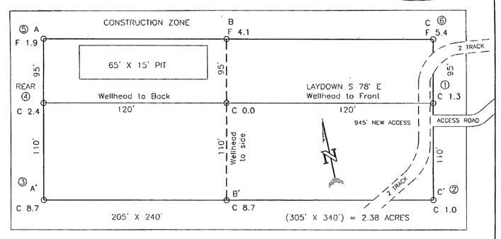
RESERVE PIT DIKE: TO BE 8' ABOVE DEEP SIDE (OVERFLOW - 3' WIDE AND 1' ABOVE SHALLOW SIDE). BLOW PIT: OVERFLOW PIPE HALFWAY BETWEEN TOP AND BOTTOM AND TO EXTEND OVER PLASTIC LINER AND INTO BLOW PIT.
