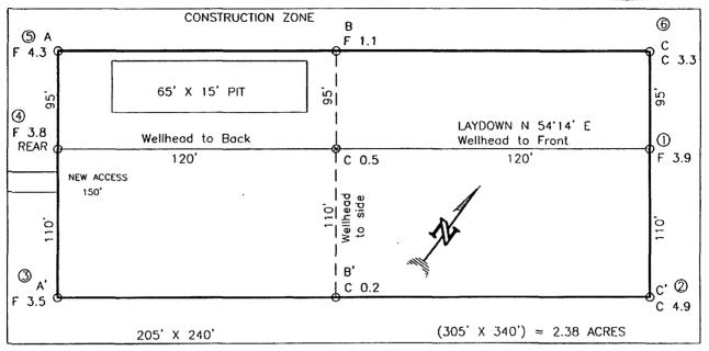
RESERVE PIT DIKE: TO BE 8' ABOVE DEEP SIDE (OVERFLOW - 3' WIDE AND 1' ABOVE SHALLOW SIDE). BLOW PIT: OVERFLOW PIPE HALFWAY BETWEEN TOP AND BOTTOM AND 10 EXTEND OVER PLASTIC LINER AND INTO BLOW PIT.
