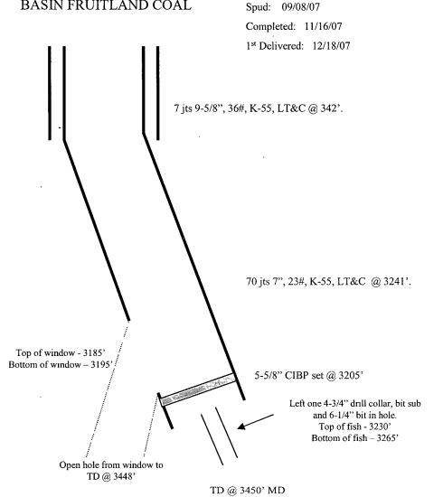
Well to be cavitated at above open hole. 5-1/2" liner and 2-7/8" production tubing will be run for production
