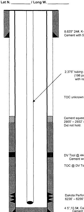
TD 6320' PBTD 6276' 8.625" 24#, K-55 Casing set @ 807' Cement with 550 sxs (Circulated to Surface)
