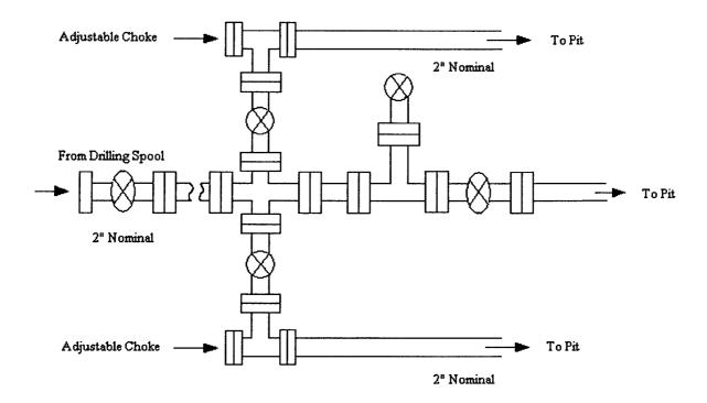
Choke manifold installed from surface to TD
