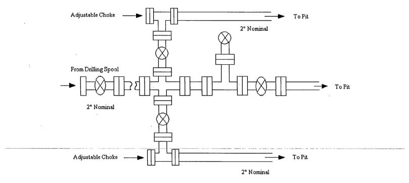
Choke manifold installed from surface to TD
