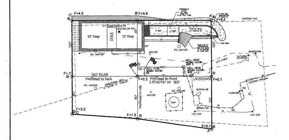
SLOPES TO BE CONSTRUCTED TO MATCH THE ORIGINAL CONTOURS AS CLOSE AS POSSIBLE.
