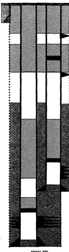
4085' TD 4075' CH PBTD 3083' PC PBTD 9.625" 32.3#, H-40 Casing set @ 125' Cement with 142 cf, circulated to surface
