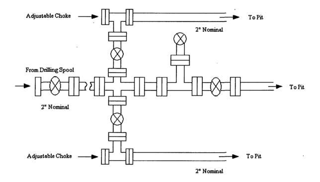
Choke manifold installed from surface to TD
