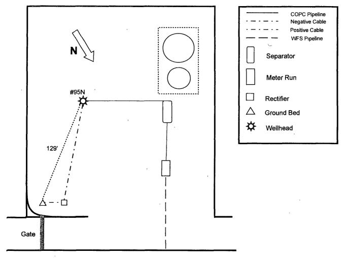
Drill ground bed approximately 129' North East of #95N wellhead at staked location. Install single well solar unit, and install cables to new ground bed and #95N wellhead at lengths below.
