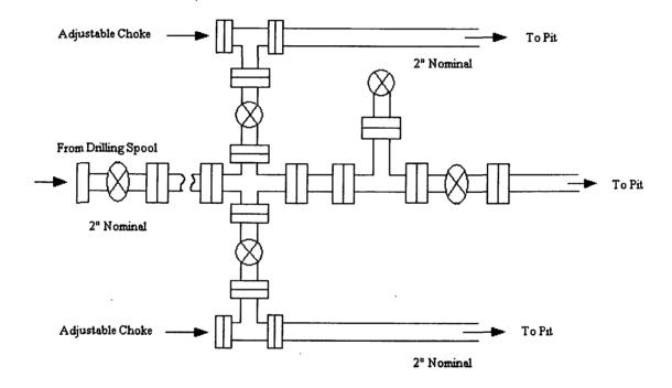
Choke manifold installed from surface to TD
