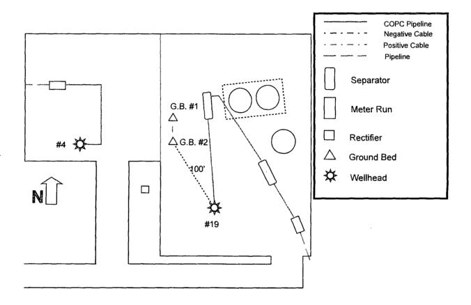
Drill new ground bed approximately 100' North West of #19 wellhead at staked location. Run new positive cable from existing ground bed #1 to new ground bed #2 at length listed below.
