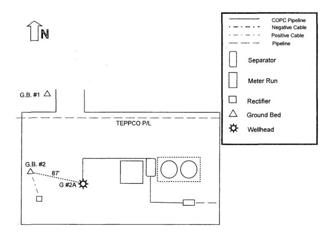
Drill new ground bed approximately 87' west of #2A wellhead at staked location. Run new positive cable from existing rectifier to new ground bed #2 at length listed below, and abandon ground bed #1 and negative wire connected to TEPPCO pipeline.
