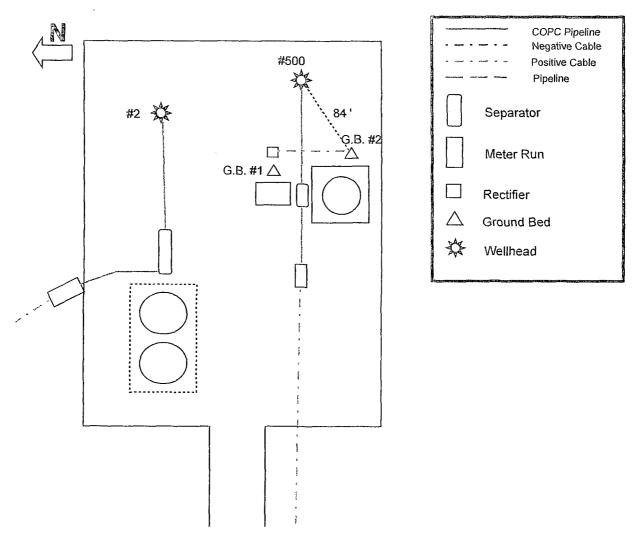
Drill new ground bed approximately 84' South West of #500 wellhead at staked location. Run new positive cable from existing rectifier to new ground bed #2 at length listed below.
