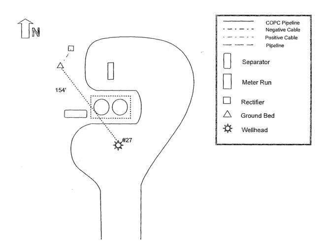
Drill new ground bed approximately 154' North West of #27 wellhead at staked location. Run new positive cable from existing rectifier to new ground bed at length listed below, and repair negative to wellhead.
