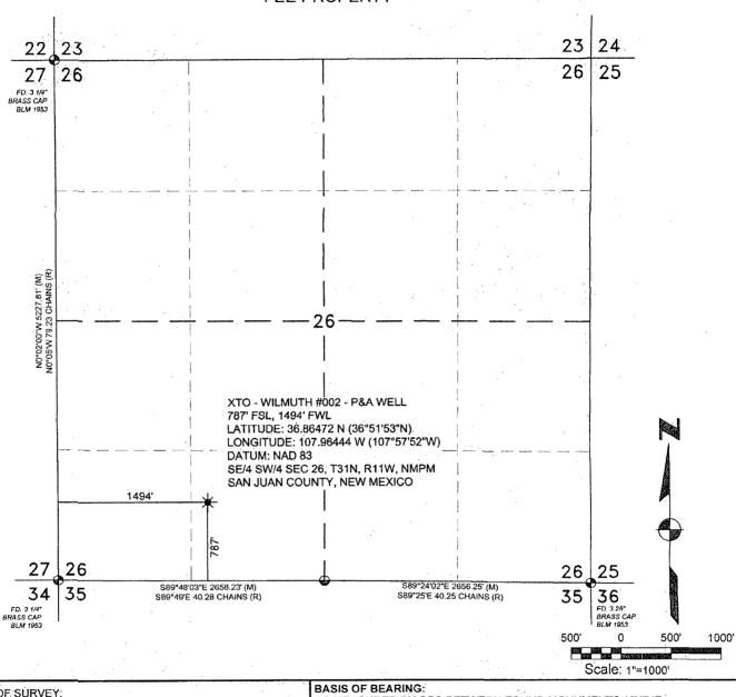
DATE OF SURVEY: AS MEASURED BY GPS BETWEEN FOUND MONUMENTS AT THE 1. 7-13-10 SOUTHWEST CORNER AND THE NORTHWEST CORNER OF SECTION 26, T31N, R11W, N.M.P.M., SAN JUAN COUNTY, NEW MEXICO. LINE BEARS S0°02'00"E, A DISTANCE OF 5227.81" I, WILLIAM E. MAHNIKE WAS DULY TO SEED SURVEYOR IN THE STATE OF NEW MEXICO HEREBY CERTIFY THAT THIS SURVEY WAS PERFORMED BY ME OR UNDER MY DIRECT SUPERVISION AND CORRECT TO JAY KNOWLEDGE AND BELIEF. VISIONS
