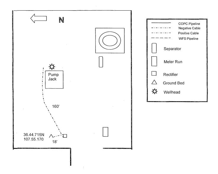
Drill ground bed approximately 156' West of #100 wellhead at staked location. Install solar rectifier at staked location. Install cable to new ground bed and to #100 wellhead at lengths below. Another well we might want to protect with this one is the Fannin #1.
