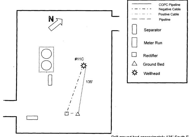
Drill ground bed approximately 135' South East of #11C wellhead at staked location. Install single well solar, and install cables to new ground bed and #11C wellhead at lengths below.
